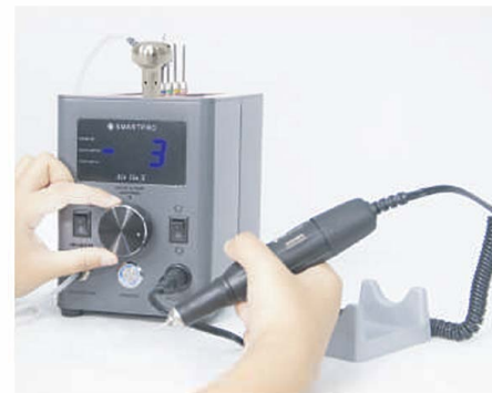
STEP 7 Adjust the control knob clockwise and counterclockwise for the desired speed level.
