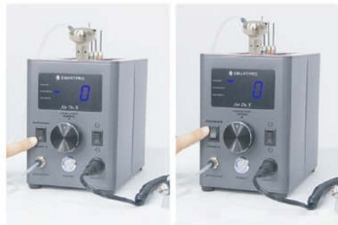
STEP 6 Tool Switching (Model-X): Select which tool to use by switching the rocker switch on left.
