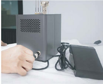
STEP 1 Connect Foot pedal at the
